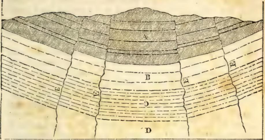
Coal basin dislocated by faults. A *Coal Measures.* B *Millstone Grit.* C *Limestone Shale.* D *Mountain Limestone.* E E E E *Faults*
